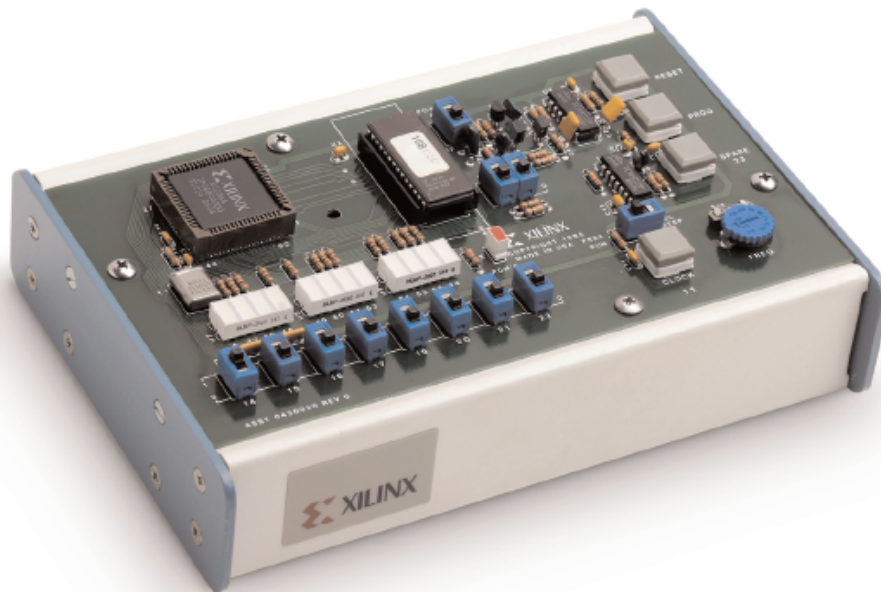
Xilinx® XC2064 FPGA Demonstration Board (circa 1985)
