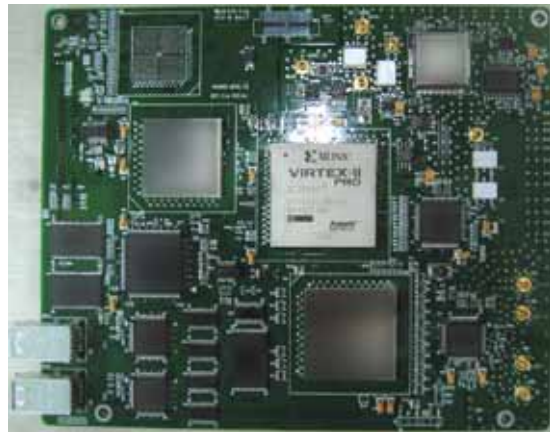
Production board for WCDMA BTS transceiver module
