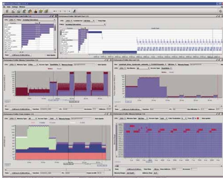
Figure 1 – Seamless FPGA's system profiler helps you tune performance by providing detailed data on bus transactions and utilization, software function execution time, bus arbitration delay, memory hot spots, and software code profiling.
