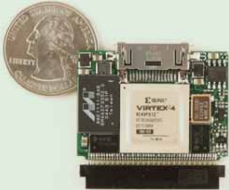
Figure 5 – The Pico Computing EP-12 card packages the FX12 or LX-25 device with a CompactFlash interface in an extremely compact form-factor.
