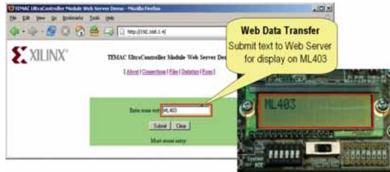
Figure 2 – Example Web server allowing remote control of ML403
