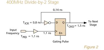
Consequently, the first stage is an unconditional divide-by-2, as shown in Figure 2. The clock-to-setup delay of 2.44 ns permits 400-MHz operation even under worst-case conditions. The flip-flop is located in the leftmost column of CLBs. This location gave the shortest route from the IOB, just 1.1ns.
