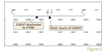
If more copies of the clock need to be driven off-chip, you should first examine the chip in EPIC to determine which I/O locations should be selected. Then, by simply adding the location constraints to your User Constraints File, and a few lines of code to your VHDL or Verilog file, you can perform the same skew analysis.
