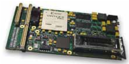
Figure 2 – AdvancedIO V1010 configurable 10GE XMC module
