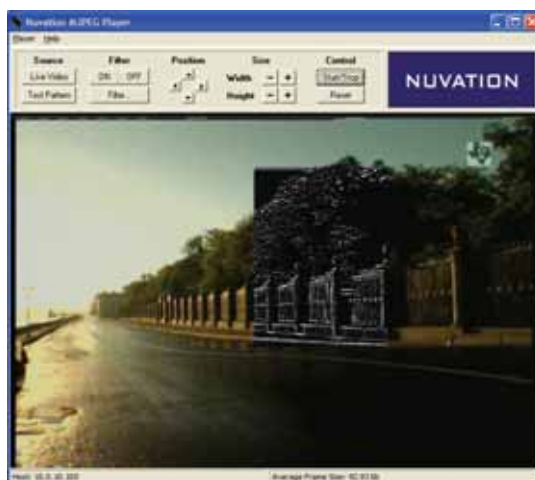
Figure 4 – MJPEG player (showing live video with edge-detect function)
