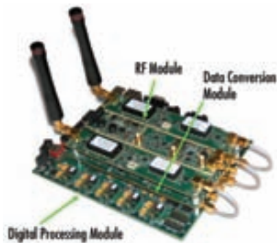
Figure 1 – The SFF SDR development platform modular platform
