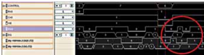
Figure 8 – 4-GHz timing analyzer memory write value and timing validation
