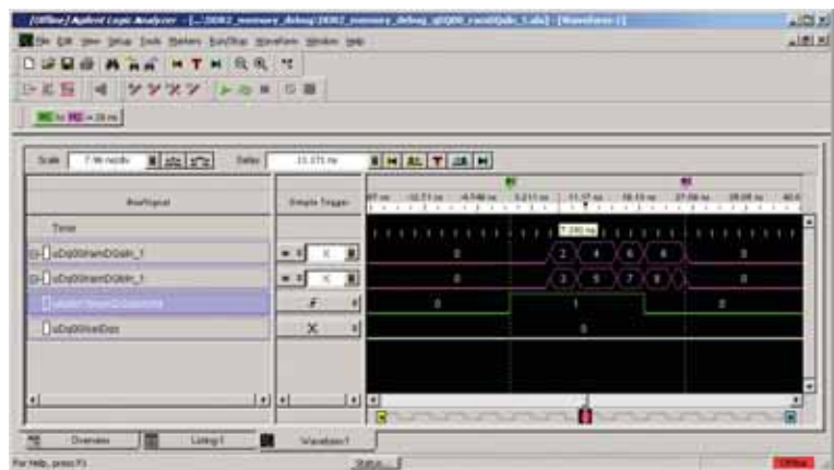
Figure 4 – Vld present one clock cycle early and misaligned to DQS A and B data
