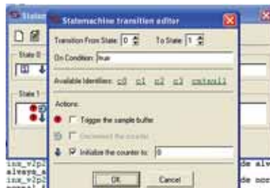
Figure 14 – The transition editor describes conditions of transitions from a state.
