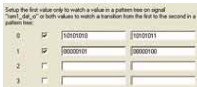
Figure 7 – The four values 0-3 indicate that the currently selected IICE was configured for state machine triggering and that the four values correspond to C0-C3 in the state editor.
