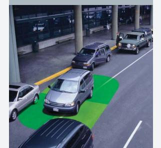
The Xilinx Automotive Targeted Design Platform for four-camera surround view provides the multi-camera support and image processing needed to stitch four images into a seamless single image with 3D multi angle view. Extensive image processing IP, image compensation for fish eye lens and camera offsets are used to provide a single matched image for parking assistance.
