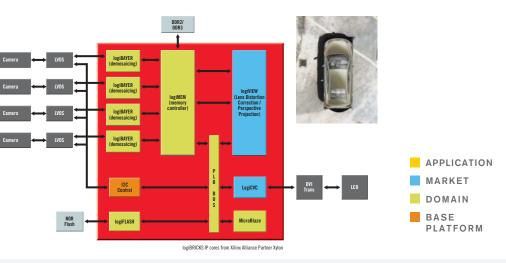
The Spartan-6 FPGA SP605 Evaluation Kit is used as the base platform for the Surround View Targeted Design Platform with an additional camera interface board connected via the FMC (FPGA Mezzanine Card) connector and four cameras.
