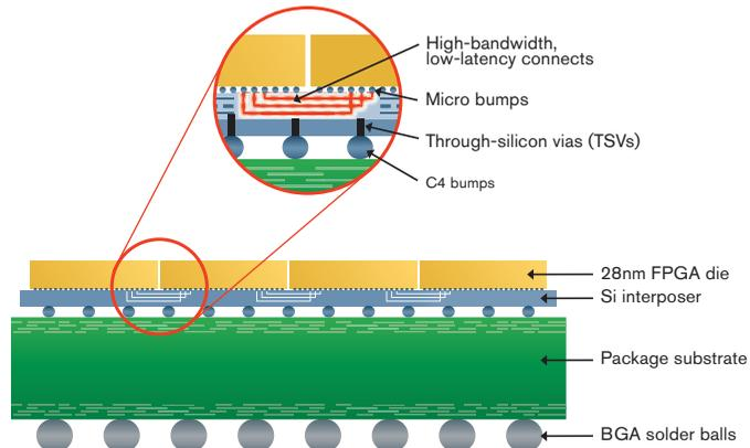
Figure 2. Schematic of package configuration
