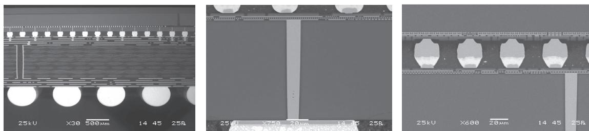
Figure 1. Cross-sections of (a) overall assembly, (b) TSV interposer, and (c)  $\mu$ bumps
