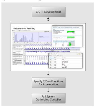
SDSoC allows users to profile their software application, using a non-intrusive profiler based on PC sampling as well as using the standard gprof profiler, to identify the function that takes up most of the time and are candidates for hardware acceleration.
