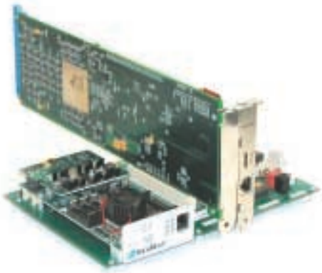
Figure 1 - PPMC750 and RC1000 connected and functioning as a prototyping platform for programmable systems
