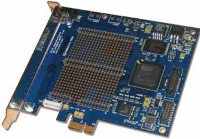
Figure 2 – The PLDA XpressLite SP3 is based on a Xilinx Spartan-3 FPGA and includes NXP's PCIe PX1012A PHY and PLDA's XpressLite IP controller.
