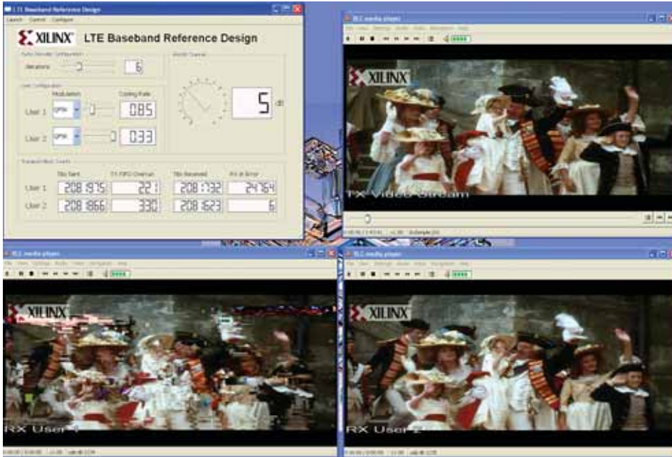
Figure 4 – Screenshot of demo running. The GUI allows variable modulation, encoding rate, and channel noise. Transmitted video is in the upper right-hand corner. Received video (with time lag for software video decode buffers) is shown for two users in the bottom half of the figure. Uncorrected errors appear as artifacts in the video decode.
