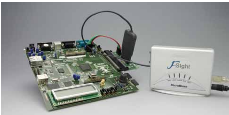
Figure 1 – F-Sight connected to a Spartan-3 board
