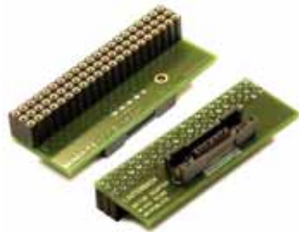
Figure 3B – Lauterbach Mictor MicroBlaze trace adapter for Xilinx MLx boards
