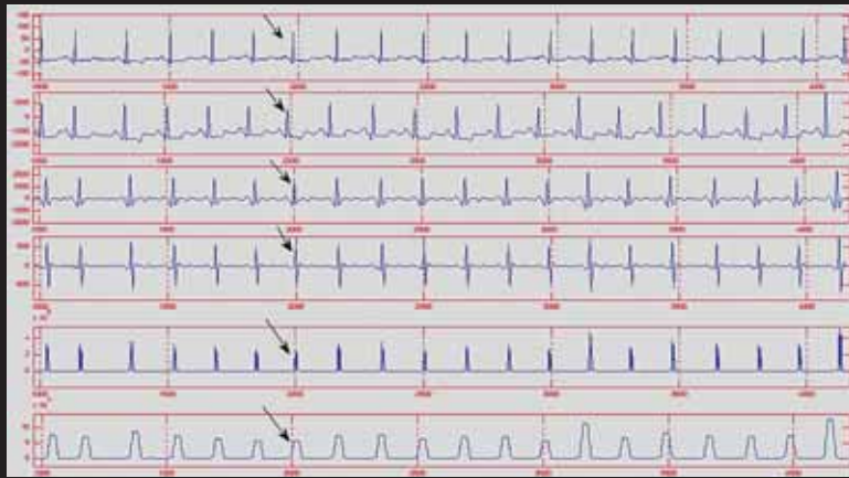
Figure 1 — Input ECG and filtering stages output, from top to bottom: original signal, low-pass output, high-pass output, derivative output, squaring stage output, moving window integrator output. The arrow indicates the position of the QRS complex.
