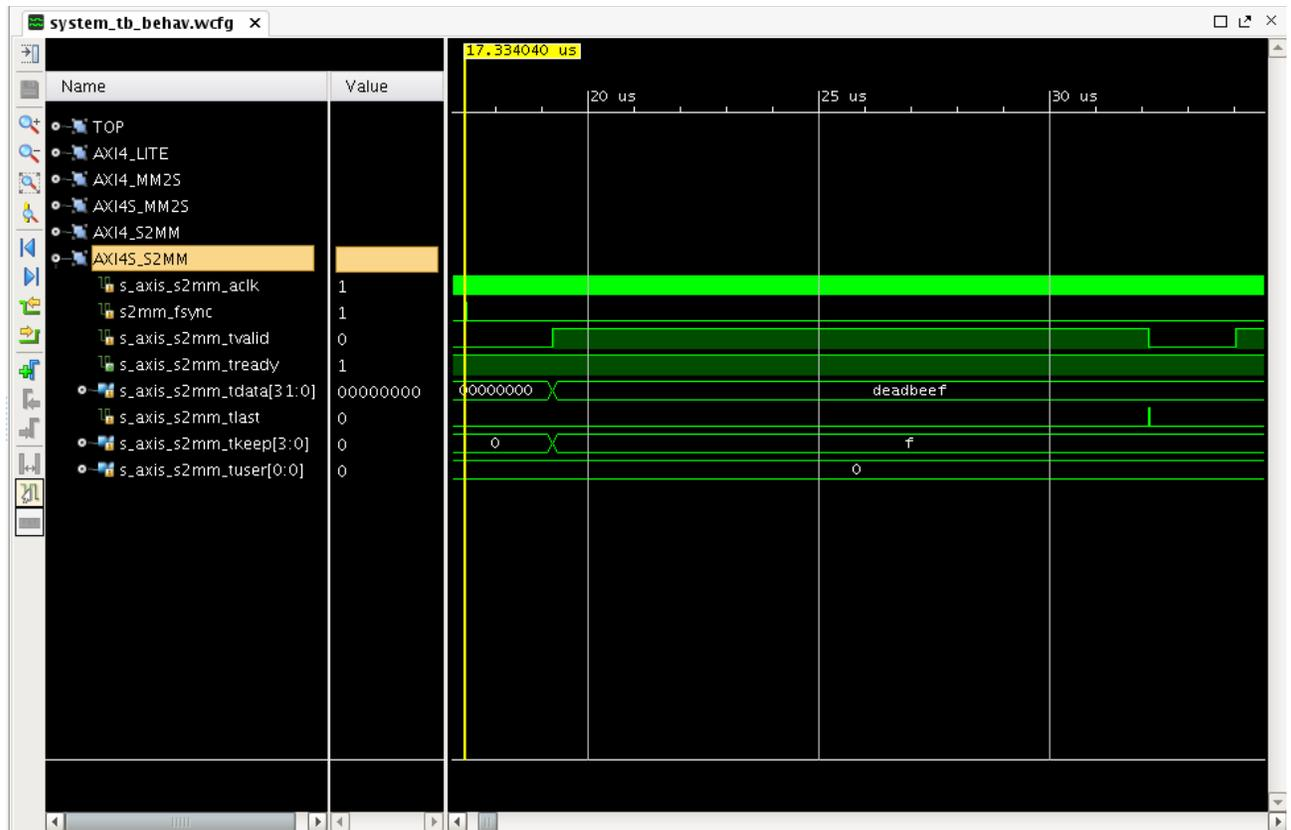
Figure 6: AXI4S\_S2MM—Horizontal Line Complete
