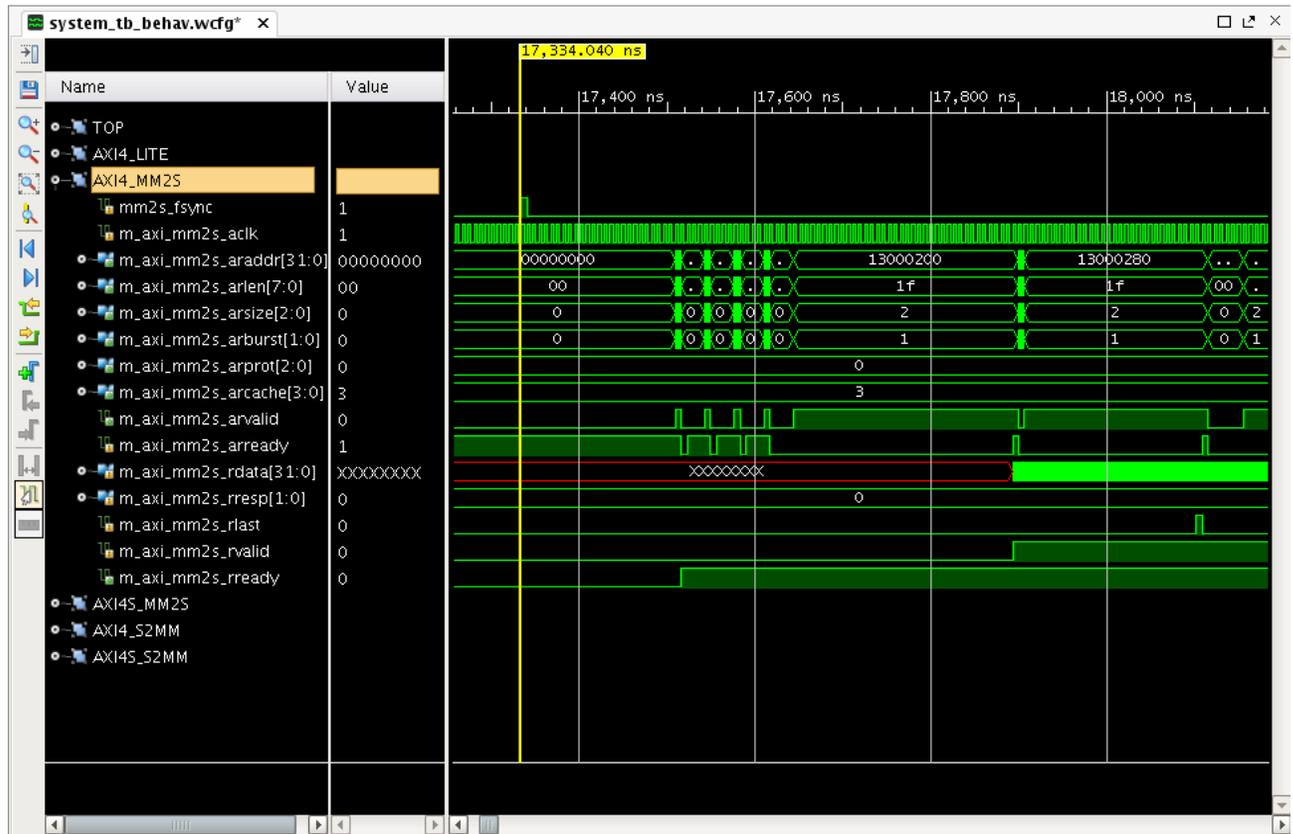
Figure 3: AXI4\_MM2S—First Reads after f\_sync
