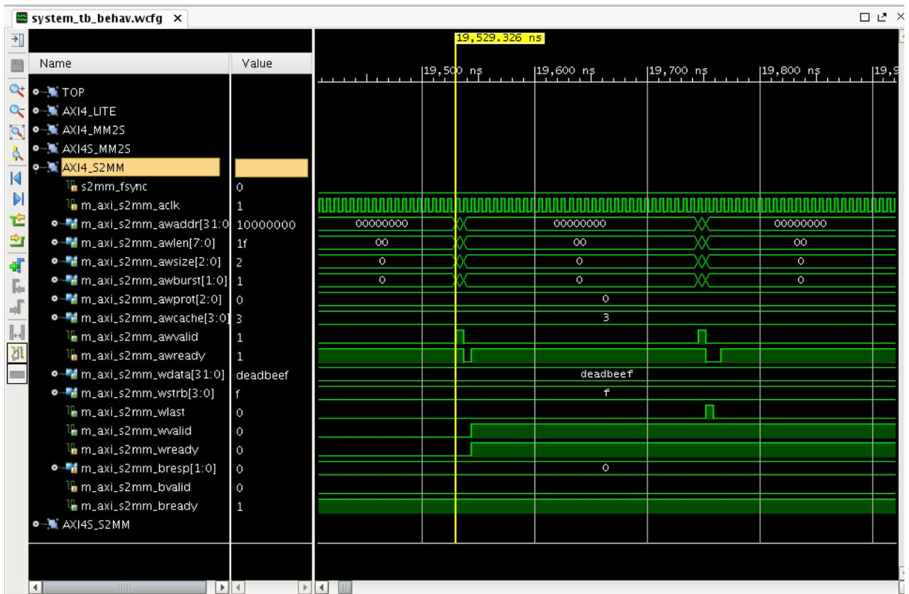
Figure 4: AXI4\_S2MM–First Write
