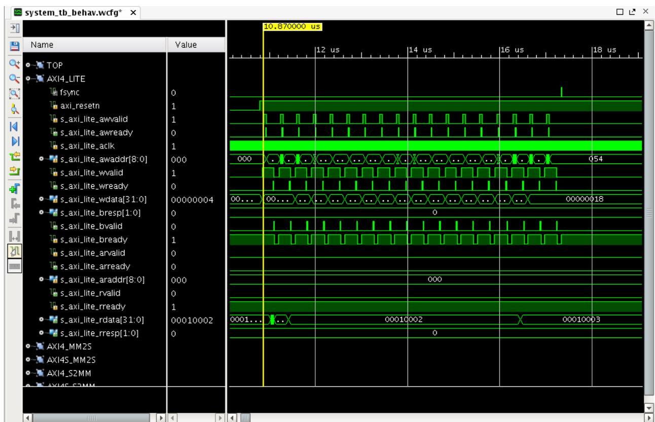
Figure 2: AXI4\_LITE–f\_sync Generated by Test Bench
