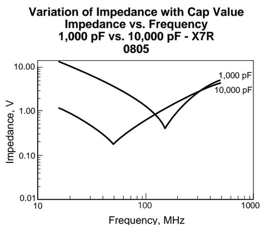
Figure 1: Capacitor Impedance vs. Frequency
