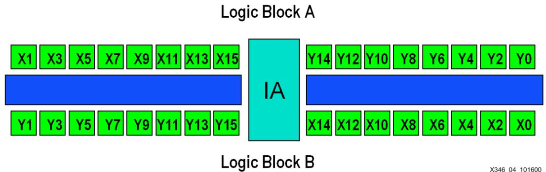
Figure 4: "Worst Case" Placement of Two Counters
