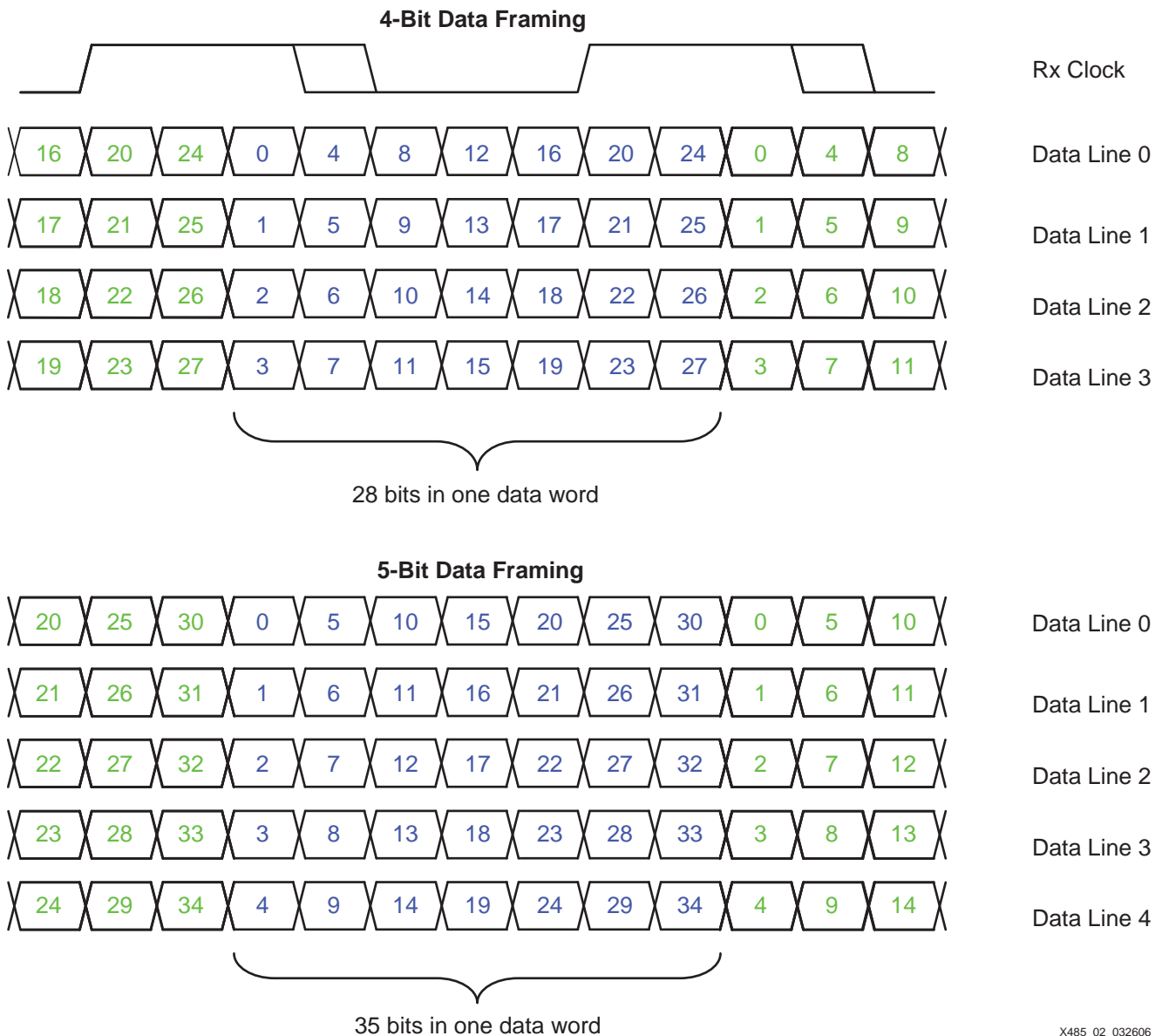
Figure 2: 4-Bit and 5-Bit Receive Data Formatting
