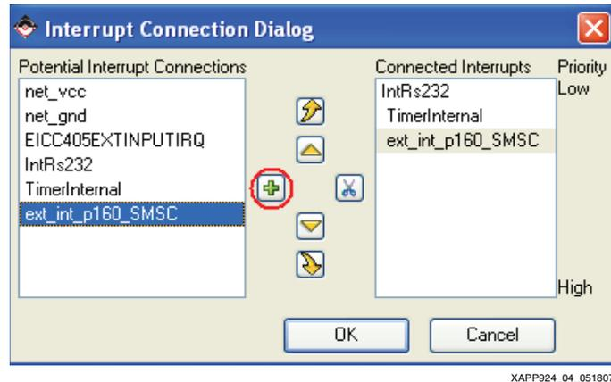
Figure 4: SMSC LAN 91C111 Controller Interrupt Signal Connection
