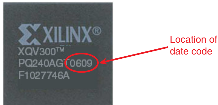
Figure 1: Package Topmark Showing 4-Digit Date Code
