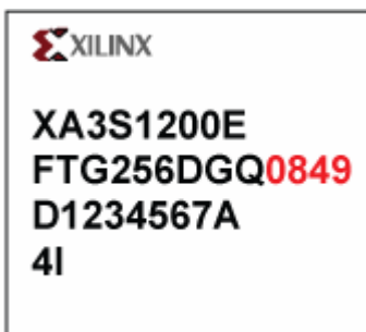
Figure 1: Example of Part Marking with Date Code (not actual date code)
