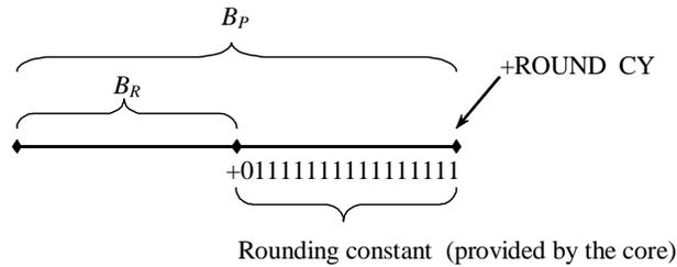
Figure 4: Rounding to  $B_r$  Bits from  $B_p$  Bits
