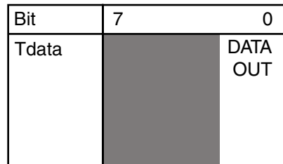
Figure 2-7: Output Data Channel TDATA Structure
