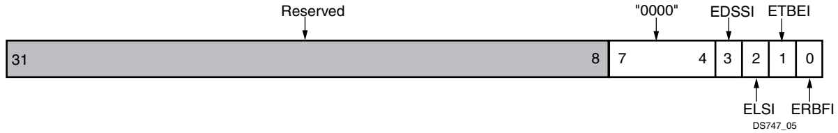
Figure 5: Interrupt Enable Register (IER)
