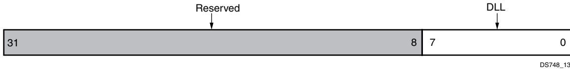
Figure 14: Divisor Latch (Most Significant Byte) Register
