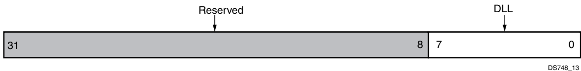
Figure 13: Divisor Latch (Least Significant Byte) Register
