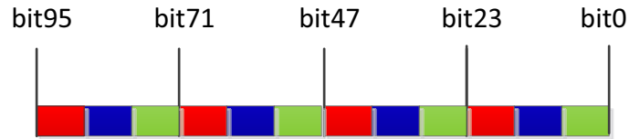
Figure 1-5: Quad Pixels RGB888
