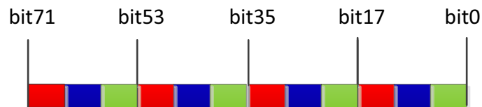
Figure 1-8: Quad Pixels RGB666 (Loosely, Packed)
