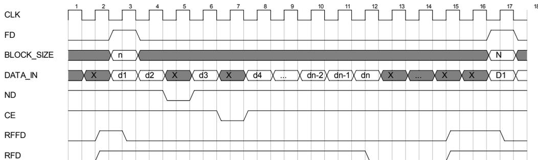
Figure 5: Input Timing
