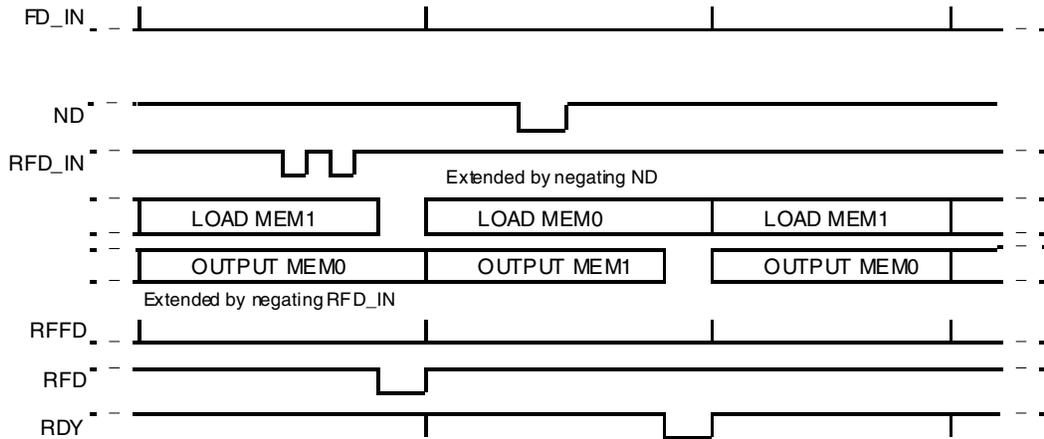
Figure 4: Double-Buffered Mode Data Throughput
