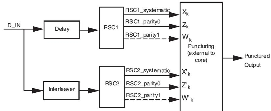
RSC1\_parity1 and RSC2\_parity1 are only available when the rate 1/5 option is selected.
