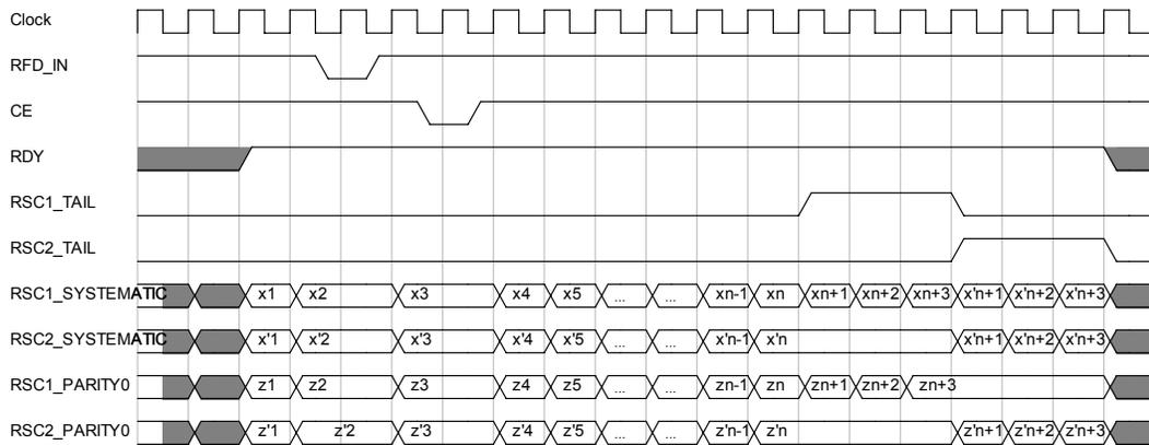
x1...xn are the uninterleaved input bits, delayed, for block size n
