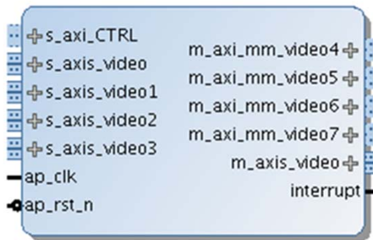
Figure 2-1: Video Mixer I/O Diagram
