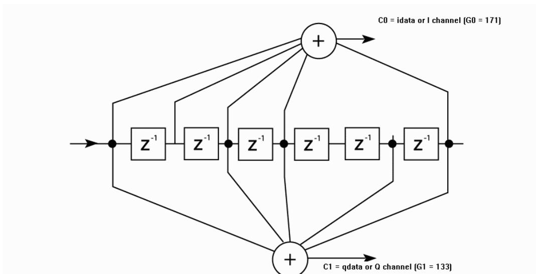
Figure 3: Convolutional Encoder of Constraint Length 7
