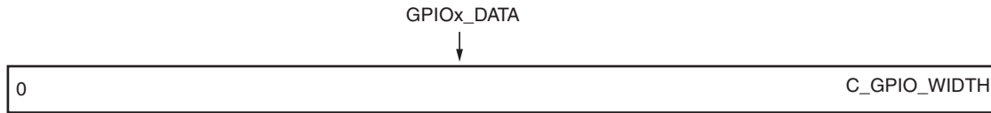
Figure 3: XPS GPIO Data Register
