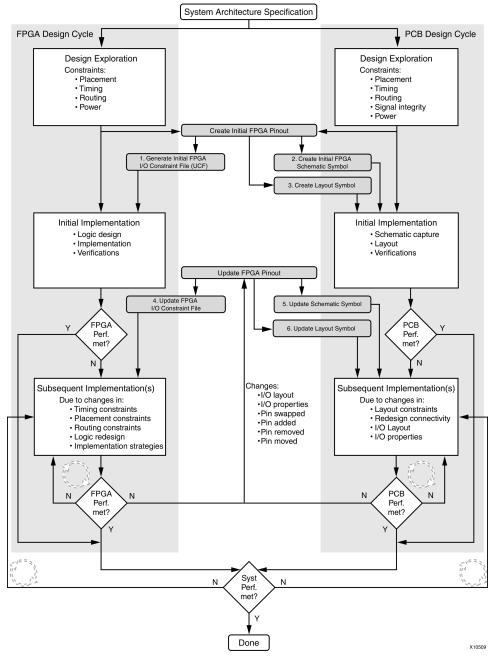
PCB design requires two main tools; namely the schematic capture tool and the PCB layout tool. These tools are described in the following sections.
