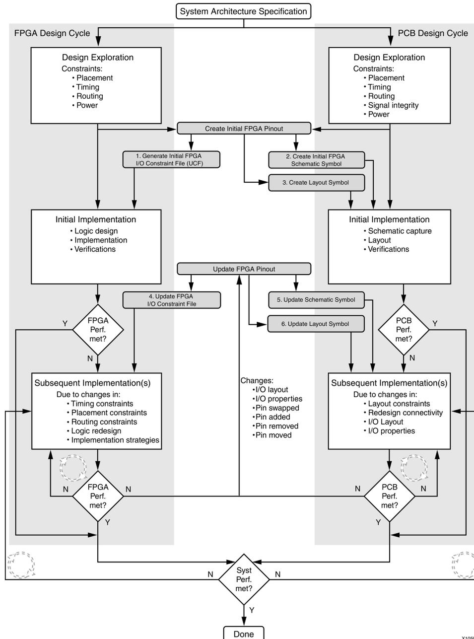
PCB design requires two main tools; a schematic capture tool and a layout tool. These tools are described in the following sections.
