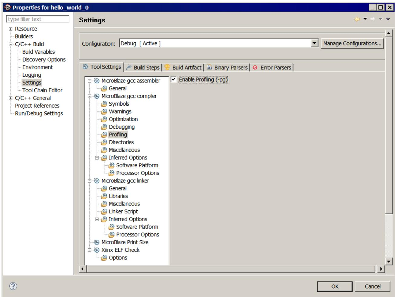
Figure 2-3: Properties Dialog Box with Profiling Enabled
