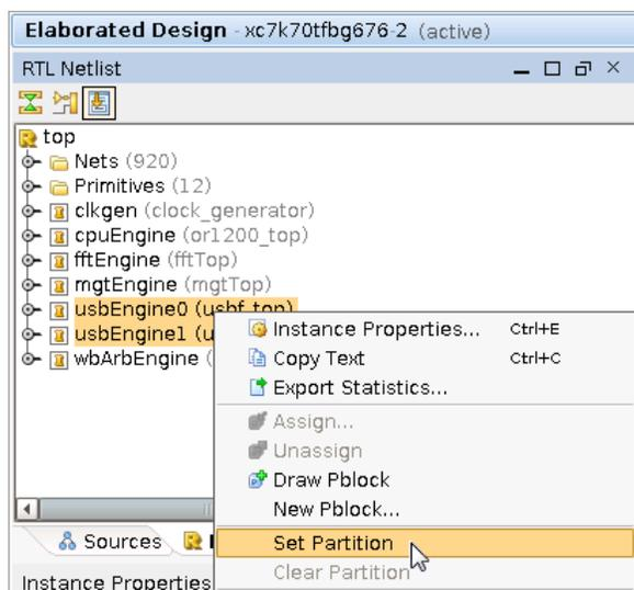
Figure 2: Setting Partitions on usbEngine Instances
