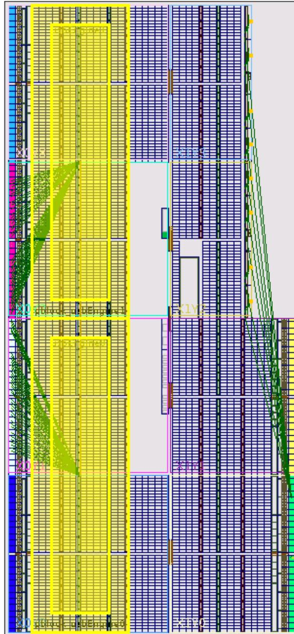
Figure 5: Completed Floorplan for Pblocks usbEngine0 and usbEngine1
