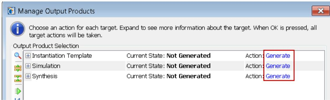
If the Generate drop down menu option is selected for the Instantiation Template, after OK is clicked, the menu will generate the .veo and related files. Pay attention to the Output product location at the bottom of the menu. These files are accessible through the IP Sources tab. Here is an example of the .veo file content.
