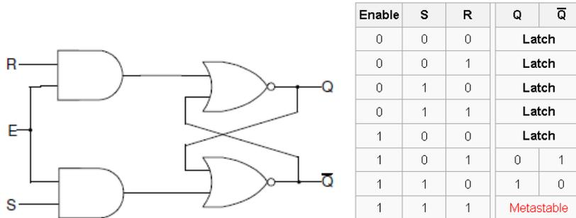
**1-2. Design a gated SR latch (shown in the figure above) using dataflow modeling. Synthesize the design and view the schematic of the Open Synthesized Design. Develop a testbench to test (generate input as shown below) and validate the design. Simulate the design. Assign S input to SW0, R input to SW1, and Enable input to SW2. Assign Q to LED0 and Qbar to LED1. Implement the design and verify the functionality in the hardware.**
