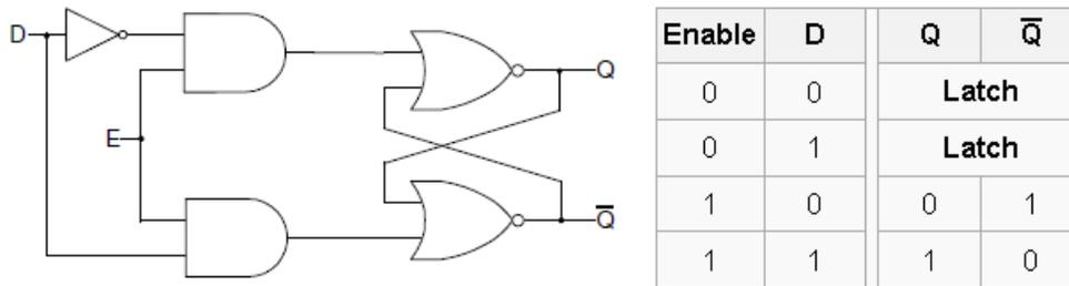
D-latches can be modeled in behavioral modeling as shown below.
