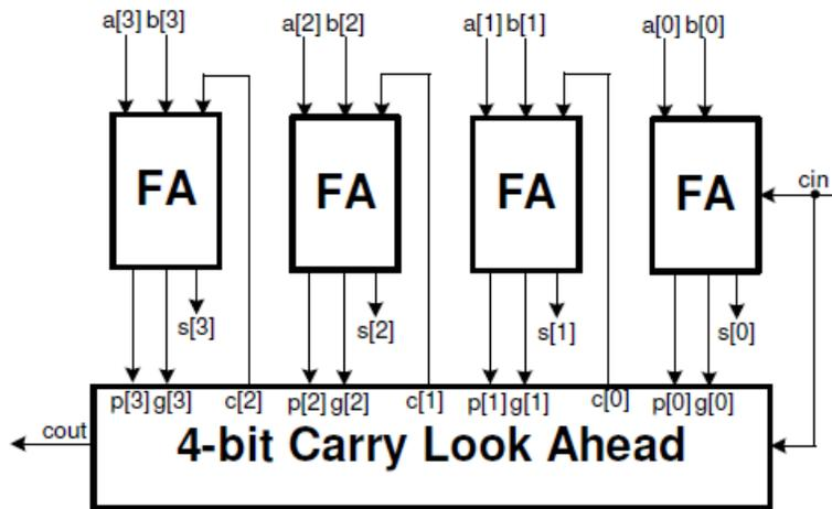
Where  $P_i = A_i + B_i$  and  $G_i = A_i B_i$ . Within Carry Look Ahead unit,  $C_{i+1} = G_i + P_i C_i$ . The speed-up is achieved through the fact that  $C_i$  being generated at the same time irrespective of  $i^{\text{th}}$  position.
