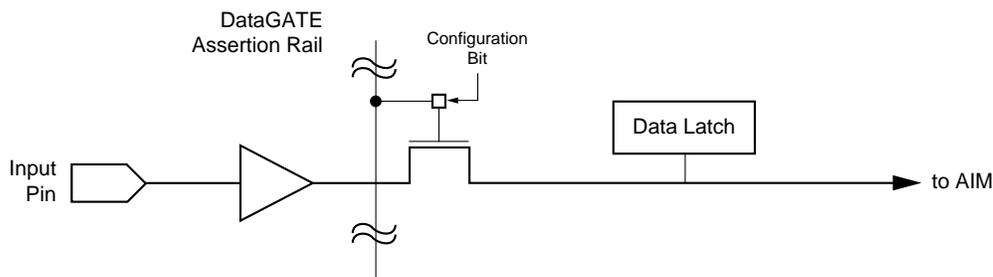
Figure 2: DataGATE Detail
