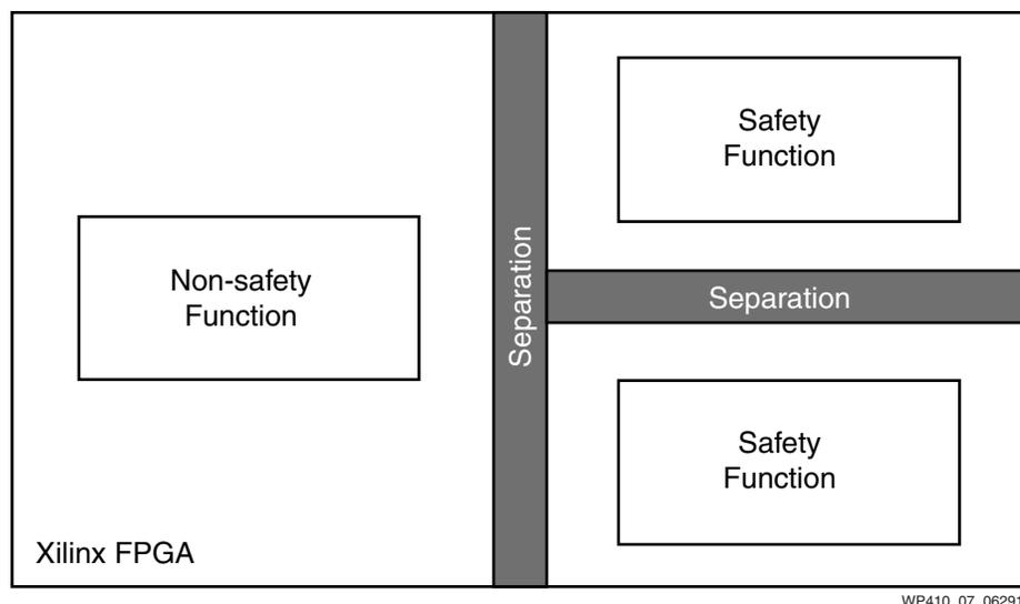
Figure 7: Xilinx FPGA Used to Implement Advanced Safety Functions
