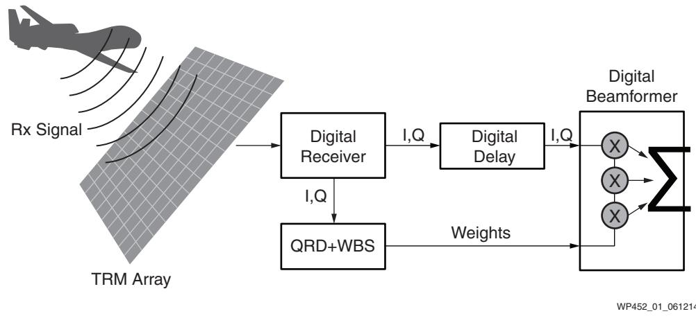
**Figure 1: High-Level Overview of Adaptive Digital Beamforming**
