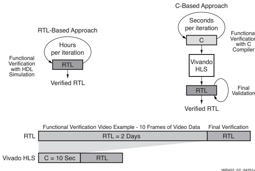
*Figure 2: RTL-Based vs. C-Based Iterative Development Time*
