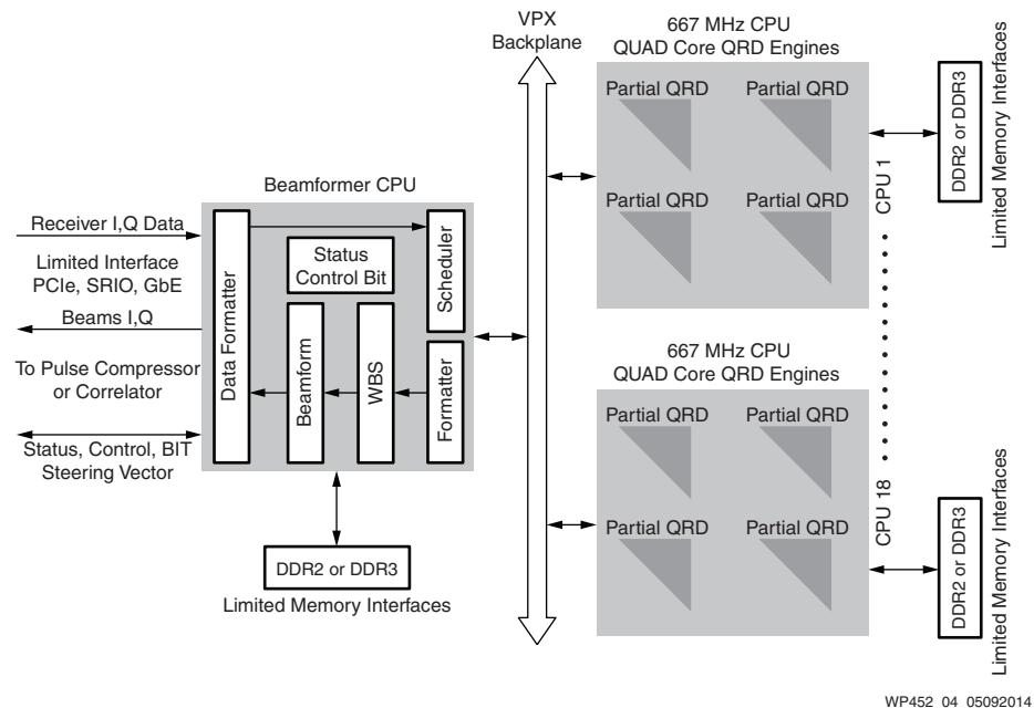
Figure 4: Adaptive Beamformer Architecture Using 18 CPUs (72 Cores)
