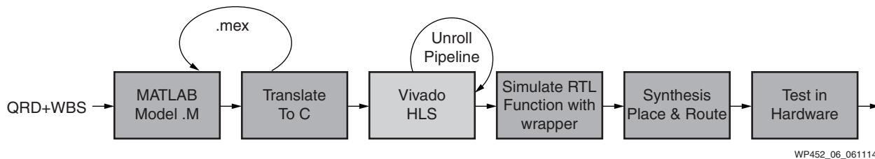
*Figure 6: Adaptive Beamformer Design Flow Using HLS*
