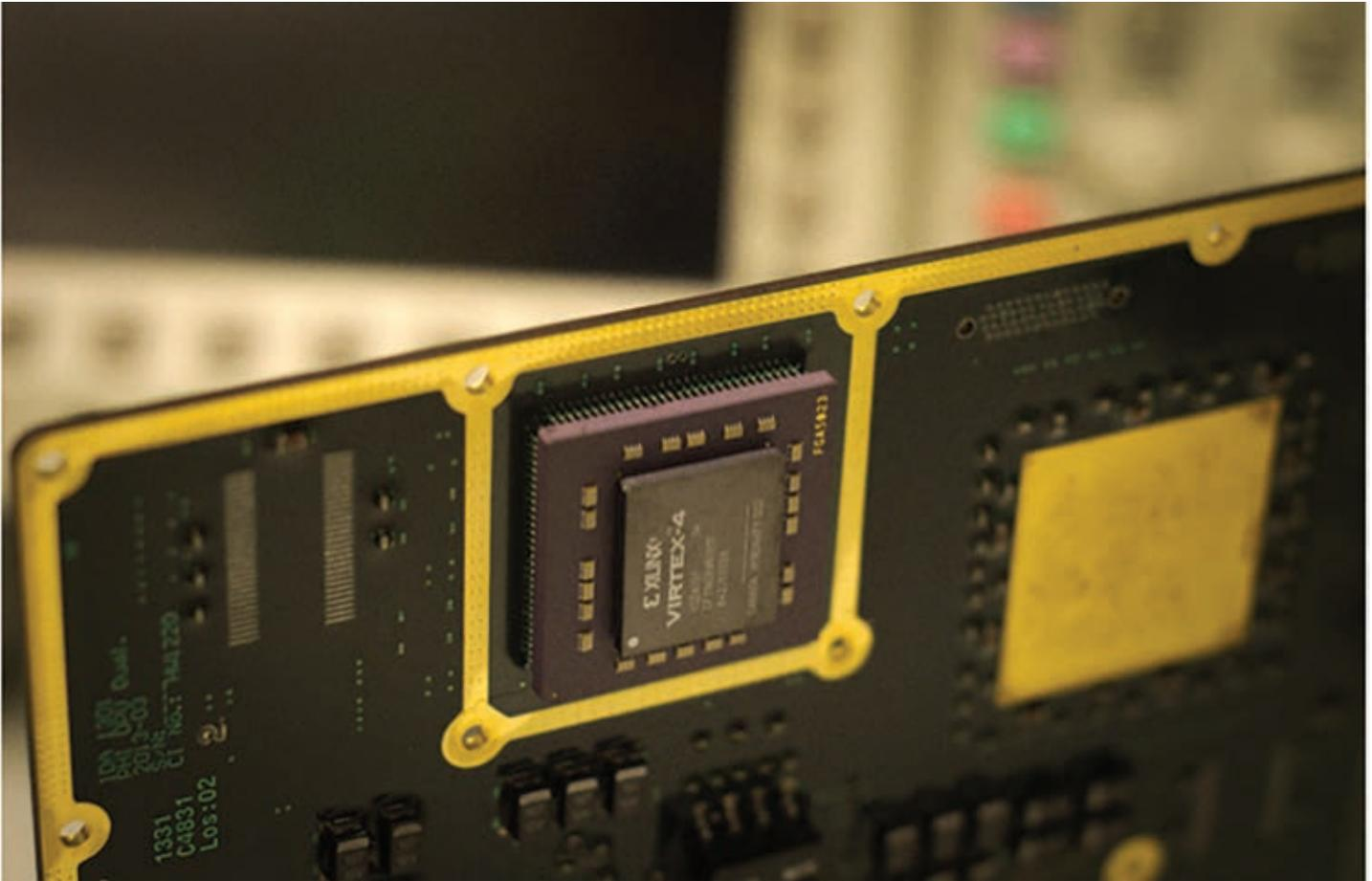
Figure 3 – Qualification board with soldered daisychain device
