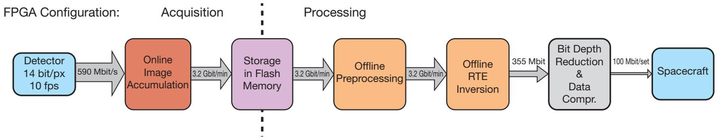
Figure 1 – Polarimetric and Helioseismic Imager (PHI) data-processing pipeline
