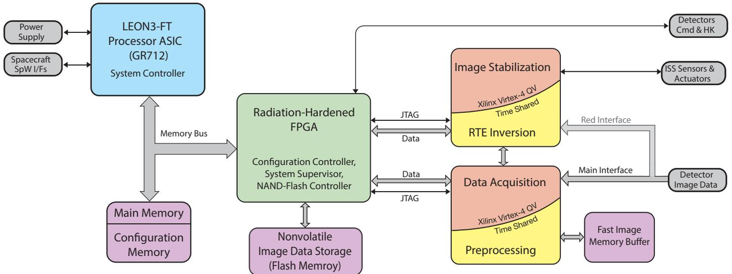
Figure 2 – Architecture of the PHI data-processing unit
