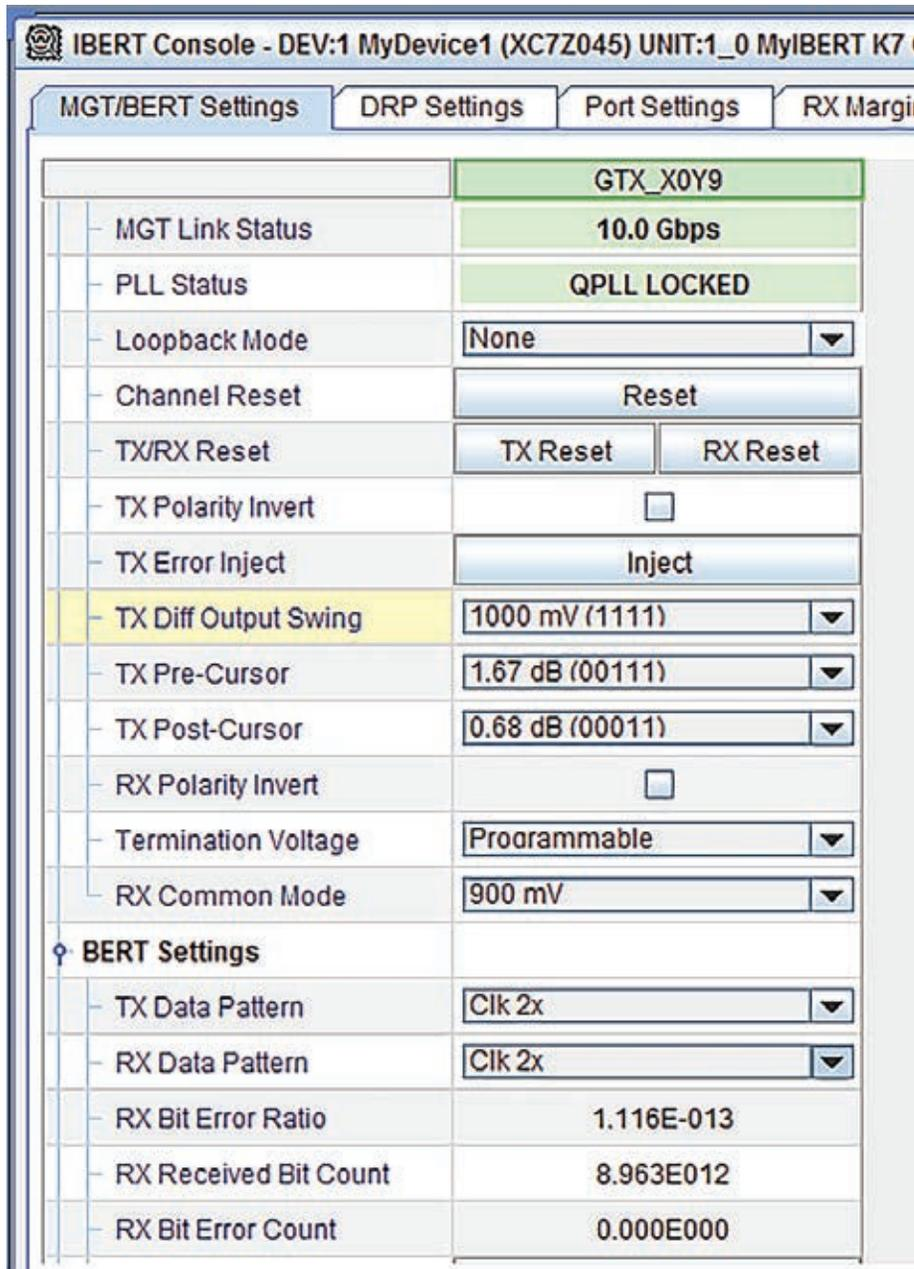
Figure 2 – Snapshot of the ChipScope Pro screen
