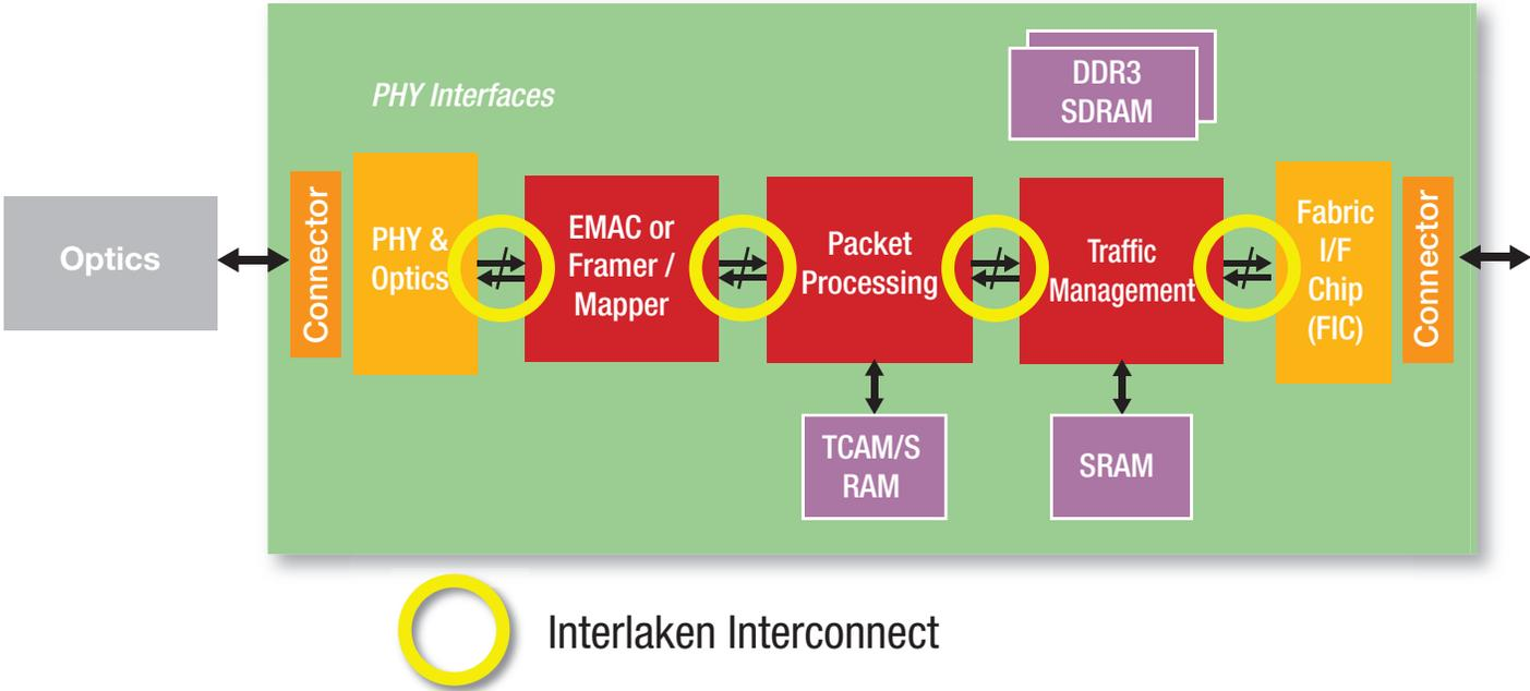
Figure 1 – Potential locations for Interlaken in packet processing
