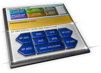
The Xilinx Zynq RFSoC DFE, a new class of product, has more hard logic than soft, but remains adaptable to address new market requirements, new services, and customer needs. This innovative approach provides twice the DFE compute resources<sup>4</sup>, is competitive with ASIC implementation on cost and power, and enables faster time-to-market.
