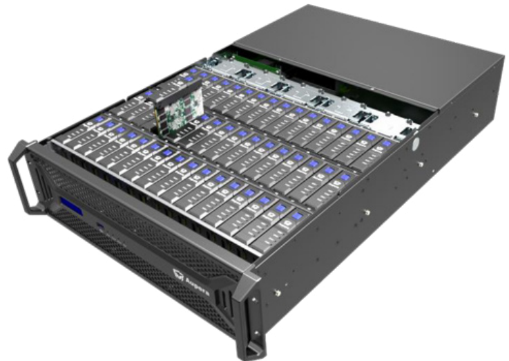
Figure 1: The Aup2600 features 48 Xilinx Zynq MPSoC devices
