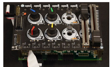
Figure 1: Hardware control for DSP implemented on a Digilent Zybo Board.
