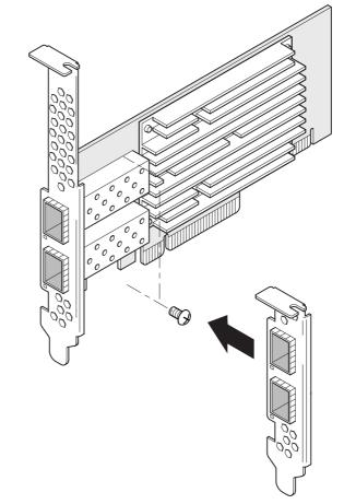
An optional 1PPS bracket and cable assembly, Solarflare part number SOLR-PPS-DP10G, is available for Solarflare dual-port SFP+ server adapters. For detailed fitting instructions, refer to the *Solarflare Server Adapter User Guide*.
